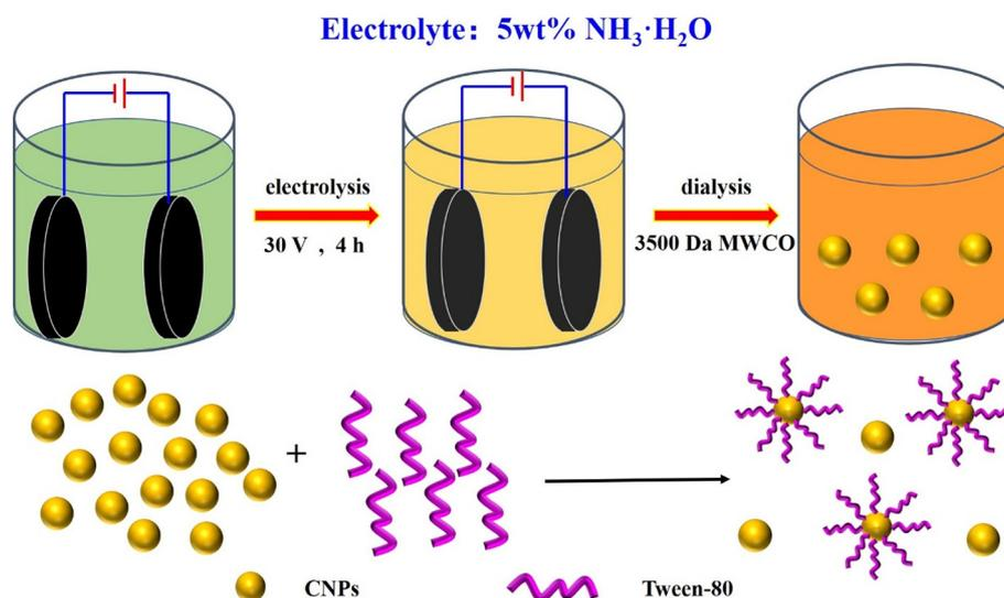
Fig. 1. The preparation process of CNPs nanofluid.
